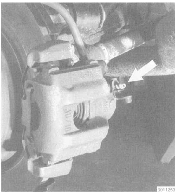
Fig. 1. Brake caliper bleeder screw (arrow).
