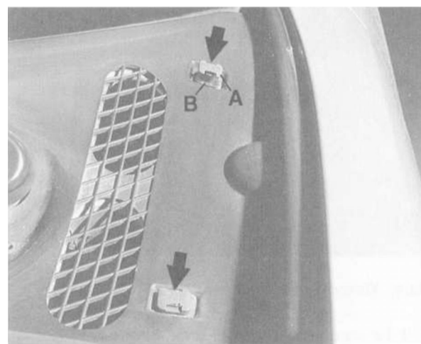
Fig. 9. Moulding grille retaining clips (arrows). Remove clip center piece (A) from outer piece (B).
