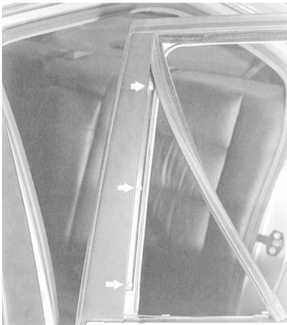
Fig. 7. Outside trim cover mounting screws (arrows). To remove cover slide up and then off door.
