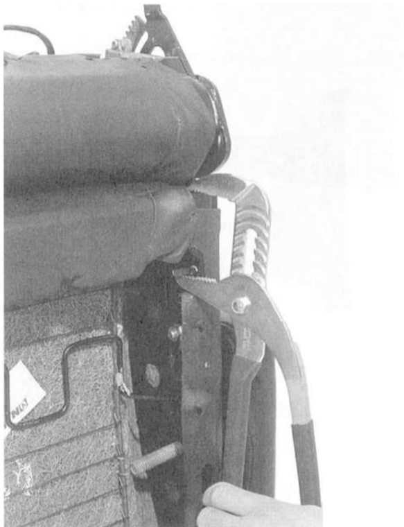
Fig. 11. Release seat back locking lever using pliers.
