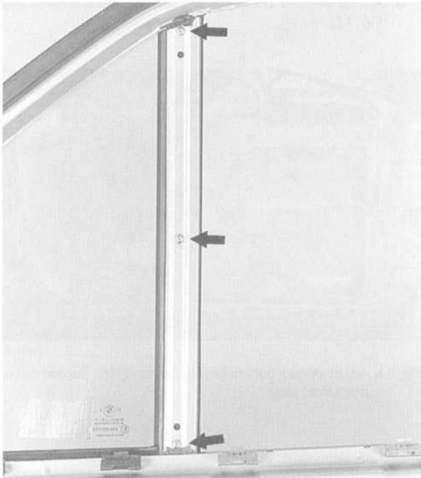
Fig. 6. Rear window guide mounting screws (arrows).
