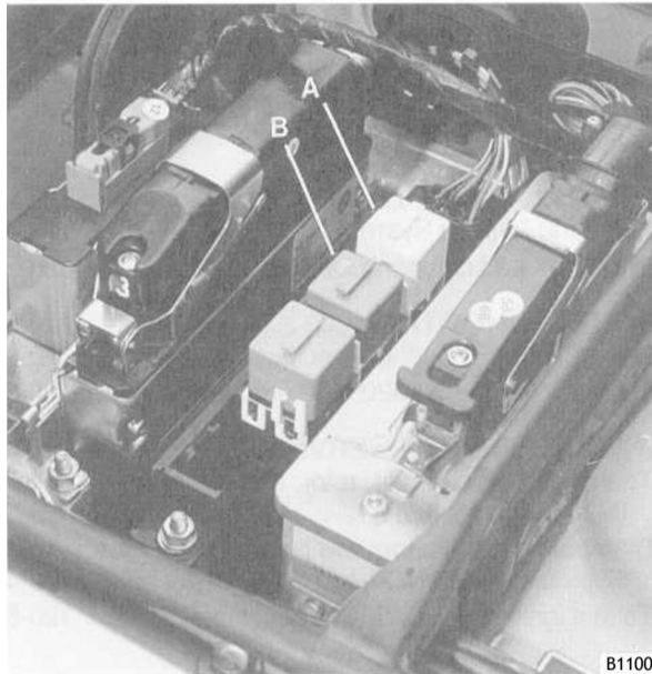
Fig. 3. DME main relay (A) and fuel pump relay (B) in right rear of engine compartment (E-Box). M50 engine shown, other engines are similar.
