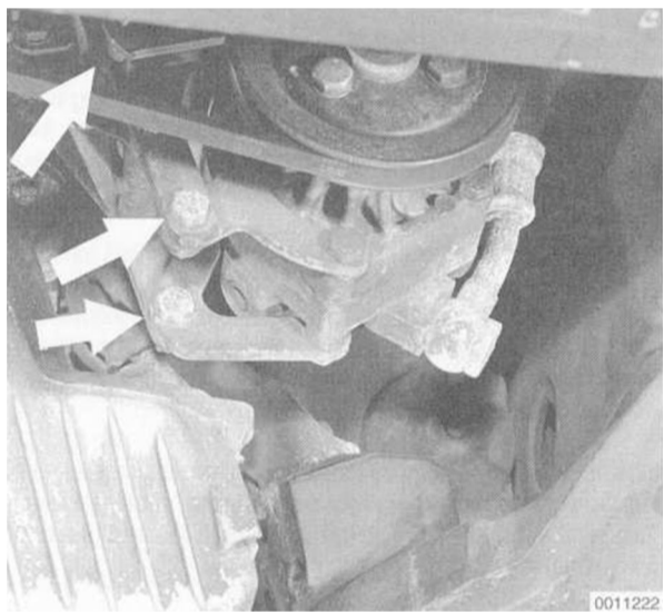
Fig. 3. Power steering pump mounting bolts (arrows) on M20 engine. Other pump mountings similar.
