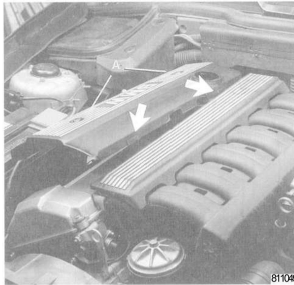
Fig. 27. Remove top engine covers by prying out caps and removing nuts (A). Note aibber gaskets at cover edge (arrows).
