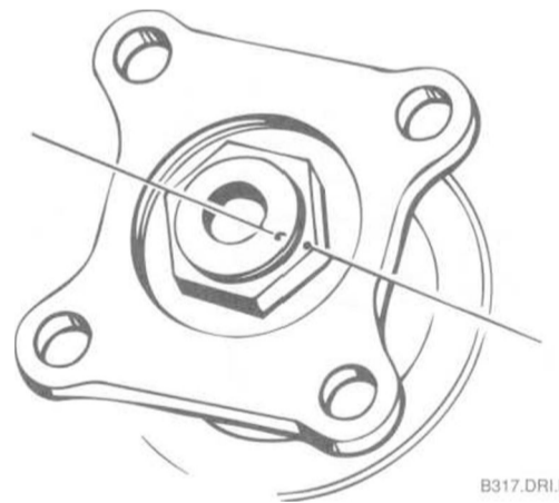
Fig. 5. Make matching marks on input shaft collar nut and flange.
