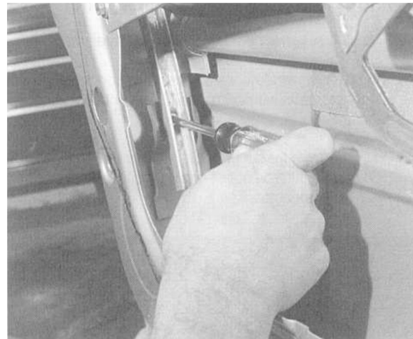
Fig. 13. Lower guide retaining bolt being removed from guide rail.
