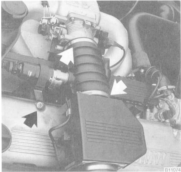
Fig. 26. Idle speed control valve (arrow).
