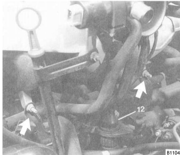
Fig. 3. Main wiring harness connector bracket under intake manifold (12). Also remove bracket mounting nuts (arrows).
