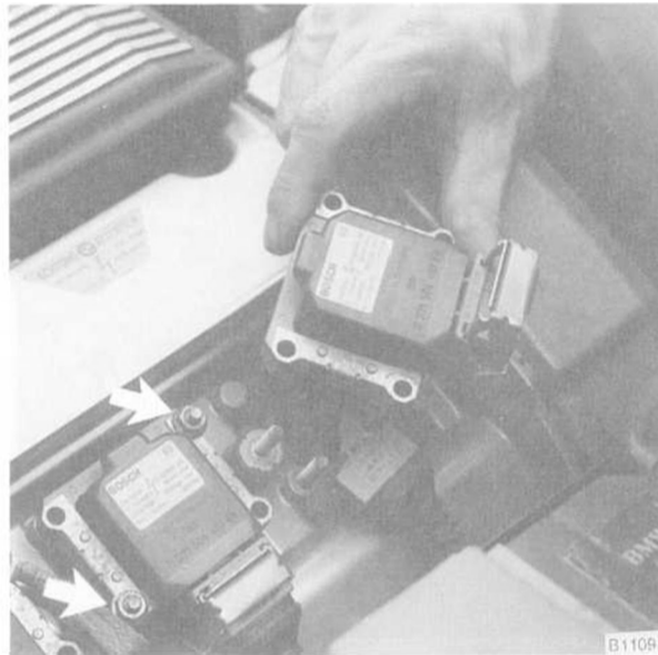
Fig. 9. Ignition coil being removed. Coil is retained by two nuts (arrows)
