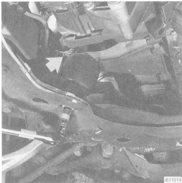
Fig. 8. Right engine mount nut being removed. Also remove ground strap (arrow).
