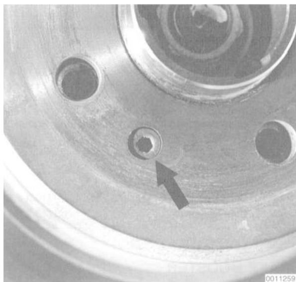
Fig. 10. Brake rotor mounting screw (arrow)
