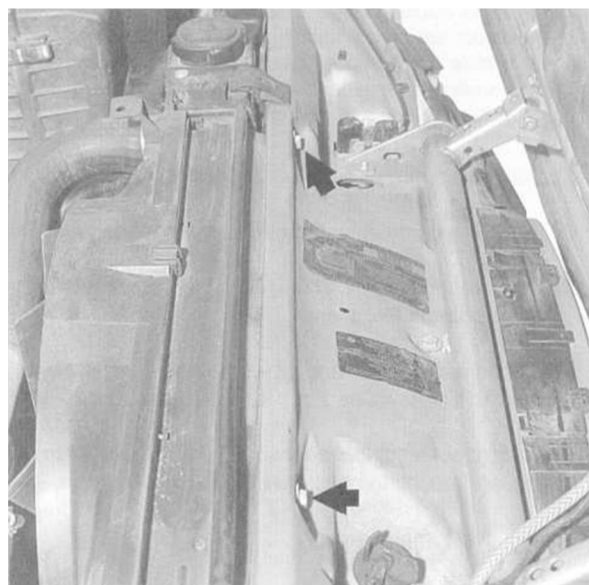
Fig. 22. A/C condenser mounting bolts on radiator support (arrows!)
