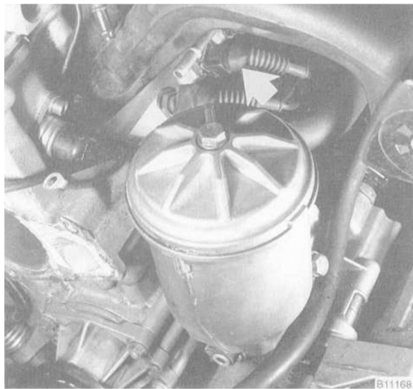
Fig. 2. Temperature gauge sender (brown body) on M50 engine. Location of sender varies depending on engine type.
