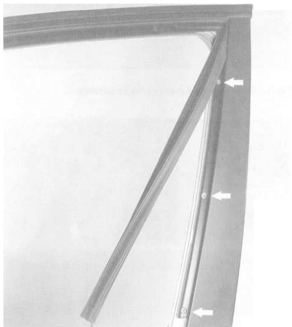
Fig. 4. Remove screws from window trim cover ( arrows ) and remove cover.
