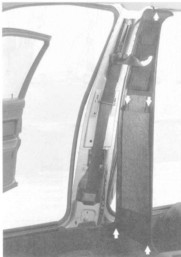
Fig. 1. B-pillar trim panel retaining clips (arrows)
