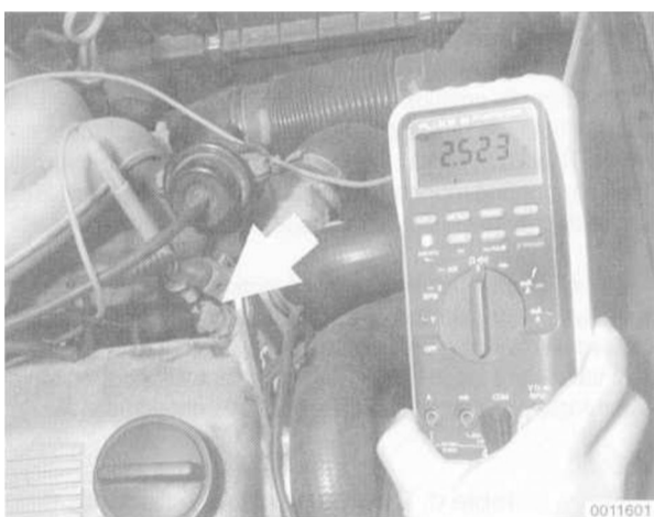
Fig. 6. ECT sensor (arrow) resistance being checked on M20 engine.
