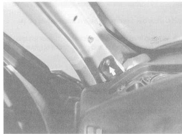
Fig. 9. Instrument panel mounting screw ( arrow ) in left side A-pillar.
