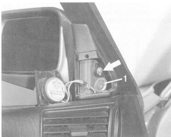
Fig. 4. Door frame trim cover mounting screw ( arrow ). Mirror mounting screw shown at (1).
