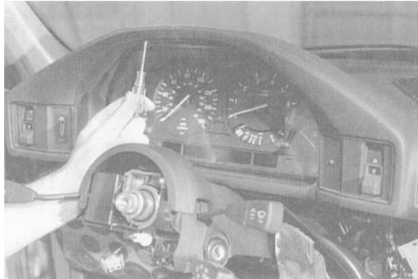
Fig. 1. Instrument cluster retaining screws being removed.
