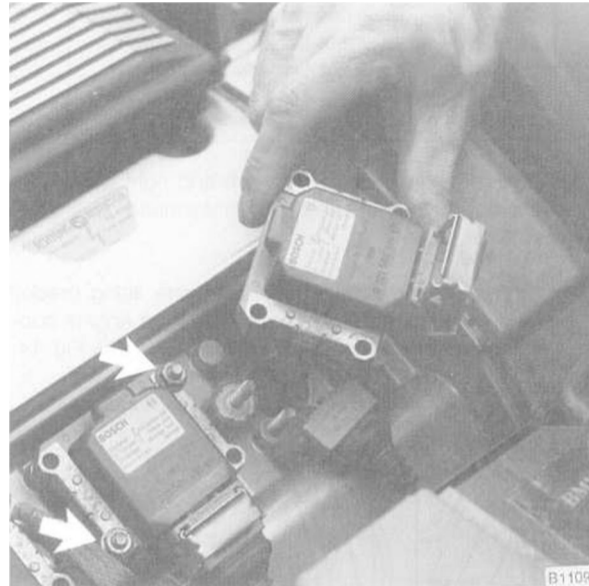
Fig. 12. Ignition coil being removed.
