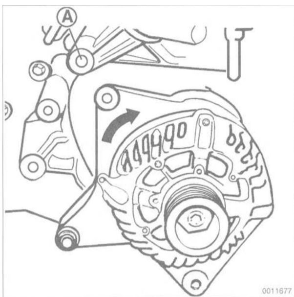
Fig. 5. On M60 engines, remove alternator by pulling oil filter housing (A) forward. Then roll alternator clockwise (arrow) under oil filter housing.
