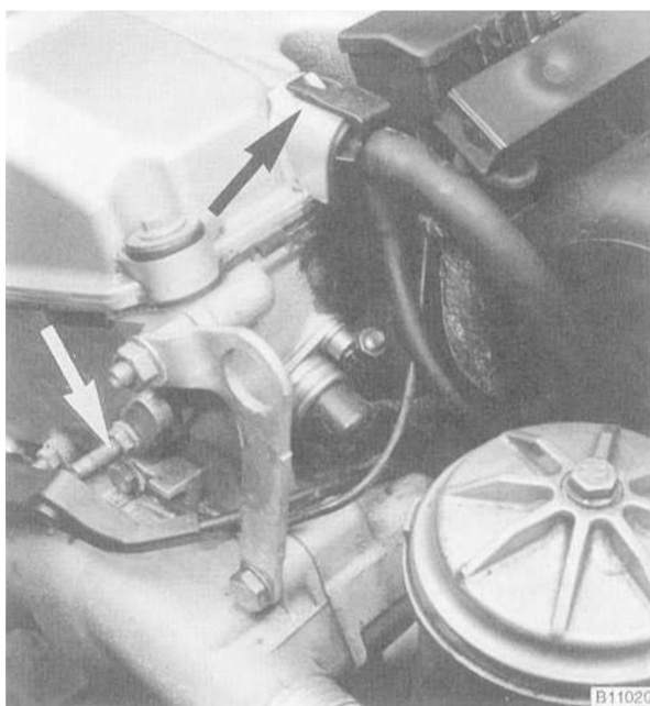
Fig. 14. Crankcase ventilation hose fitting and ground wire (arrows) to be disconnected and removed.
