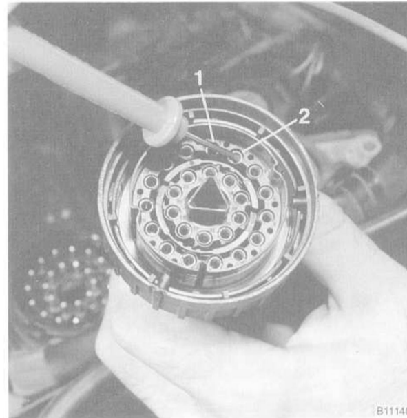
Fig. 3. Oil level sensor being tested through main harness connector. Blue/yellow wire (1) is for dynamic switch and blue/white wire (2) is for static switch.
