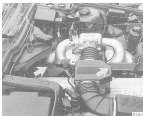
Fig. 29. Wiring harness bracket cover plugs (arrows).
