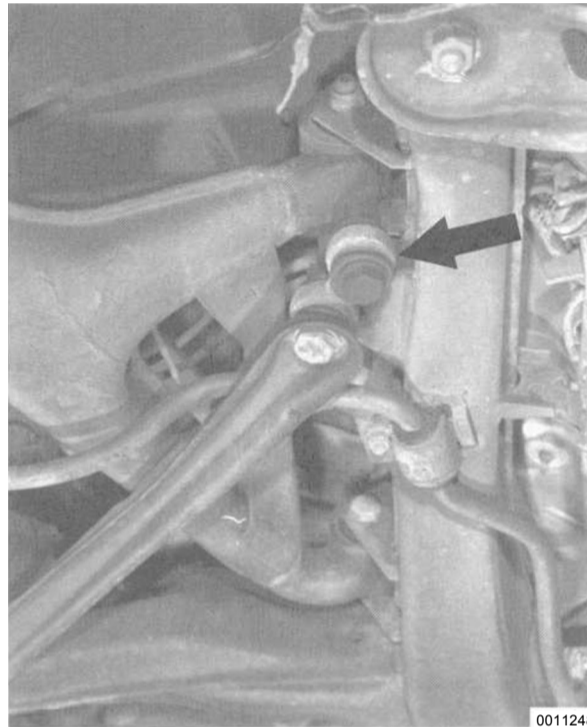
Fig. 14. Trailing arm connecting link ( arrow )
