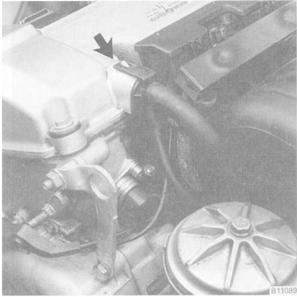
Fig. 7. Crankcase ventilation hose fitting to be removed (arrows)
