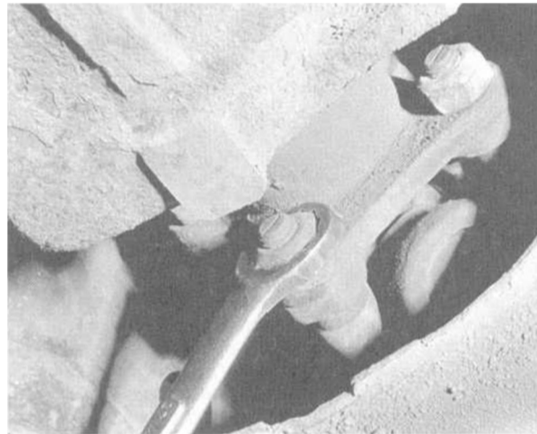
Fig. 5. Rear driveshaft to final drive mounting nut being removed.
