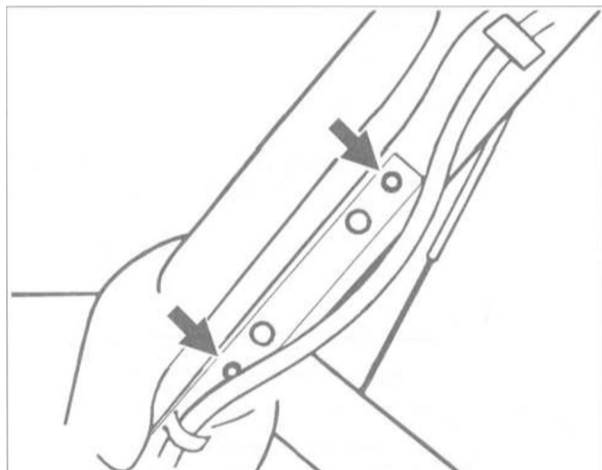
Fig. 11. Tailgate holder screws ( arrows ). Move hose aside to access
