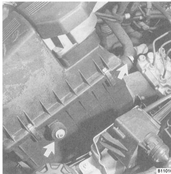
Fig. 4. Air cleaner housing mounting nuts (arrows). Loosen nuts and lift out housing.
