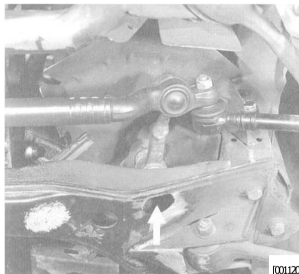
Fig. 18. Steering idler arm mounting bolt (arrow).
