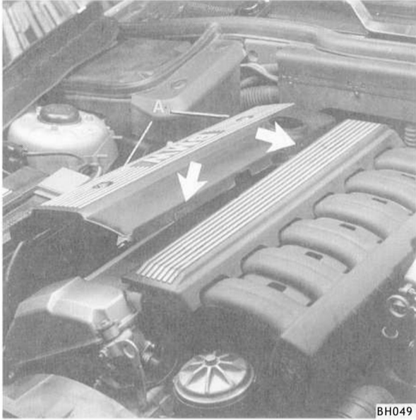
Fig. 10. Remove top engine cover by prying out plugs and removing nuts (A). Make sure rubber insulators on either side of cover do not fall off during cover removal (arrows).
