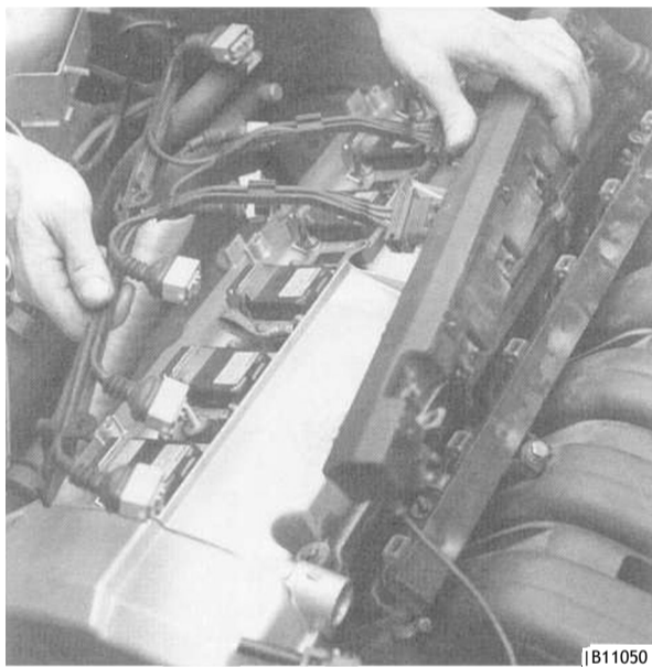
Fig. 21. Injector wiring harness duct being removed from M50 engine.
