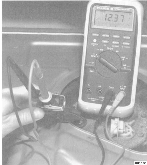
Fig. 9. Voltage supply to fuel pump being checked at harness connector terminals 4 (-) and 5 (+).
