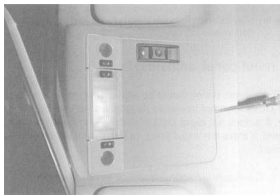
Fig. 2. Sunroof panel access cover being removed.
