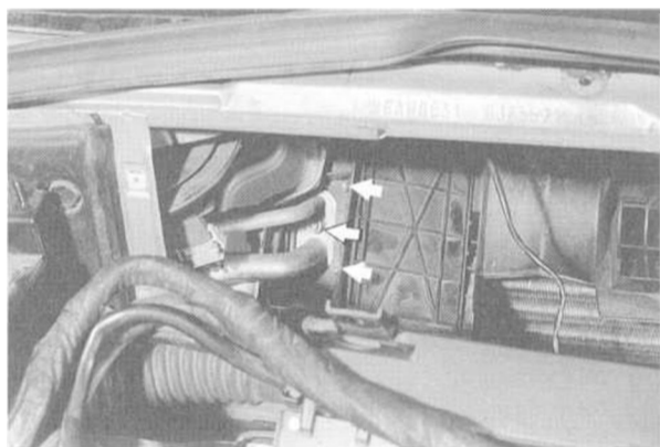
Fig. 24. Expansion valve refrigerant lines mounting nut and screws (arrows).
