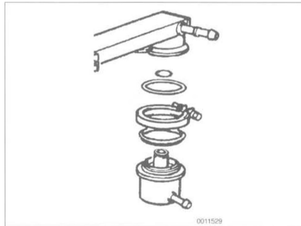
Fig. 25. Fuel pressure regulator ring clamp on 1991-1993 M50 engine. Later M50 and M60 engines use locking ring to retain fuel pressure regulator.
