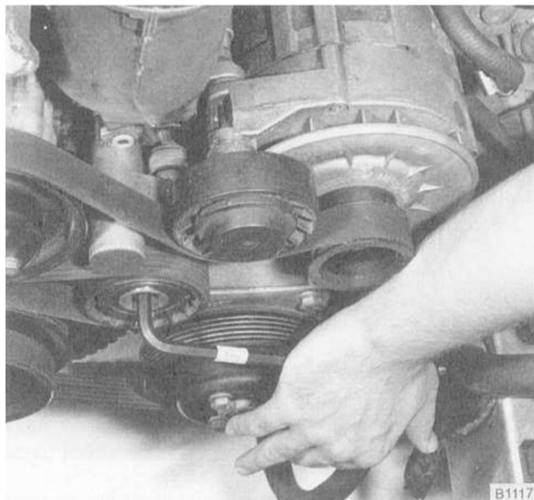
Fig. 12. Poly-V belt tensioner being released. Pry off tensioner cover and then lever tensioner clockwise to release belt tension.
