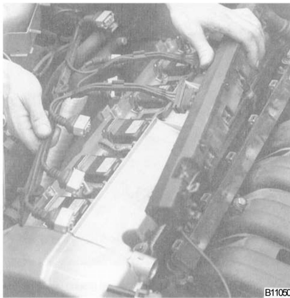
Fig. 11. Main harness being lifted off engine to be placed at base of windshield.
