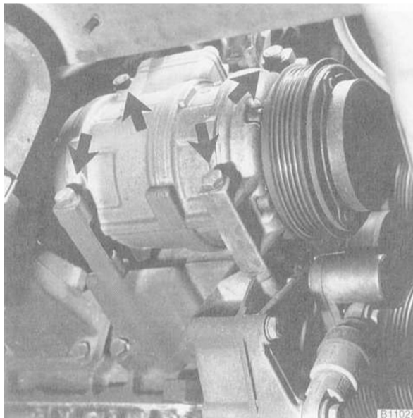
Fig. 22. A/C compressor mounting bolts (arrows)
