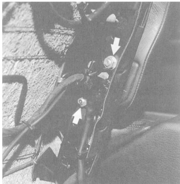
Fig. 4. Front seat armrest mounting nuts ( arrows ;
