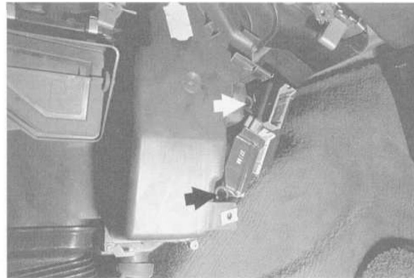
Fig. 7. Final stage mounting screws (arrows) (IHKR I and IHKA only).
