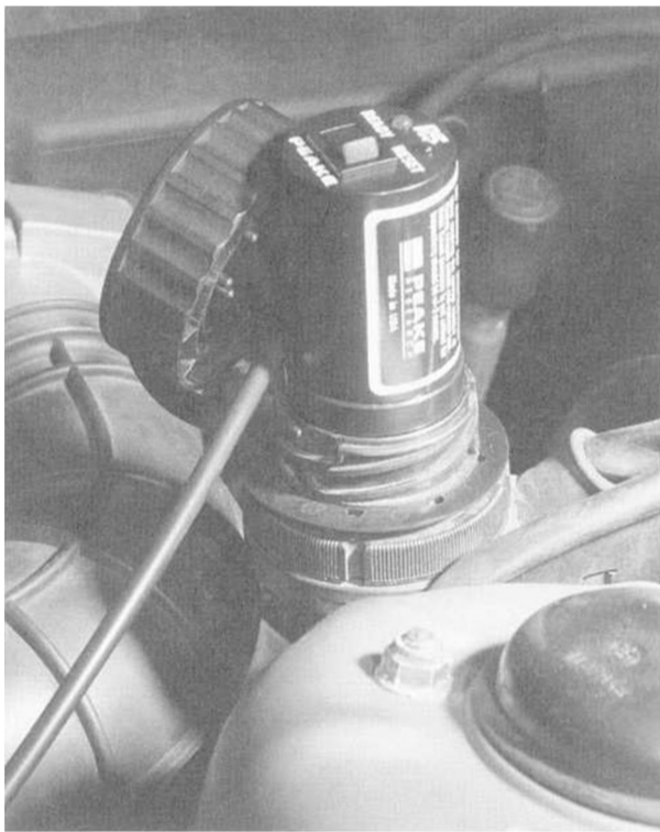
Fig. 2. Service indicator reset tool installed in diagnostic connector (aftermarket tool shown).
