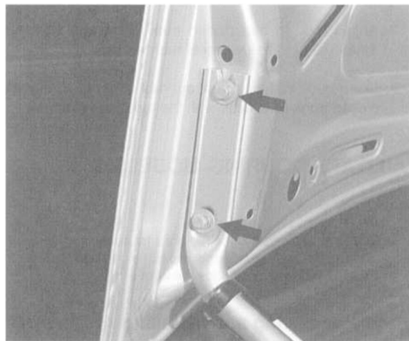
Fig. 2. Trunk lid hinge bolts (arrows). Loosen upper bolt and remove lower bolt.
