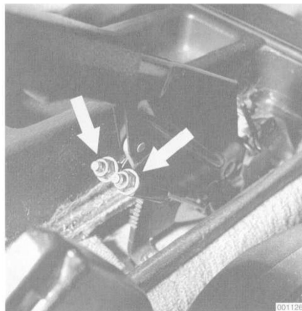
Fig. 16. Parking brake cable adjusting nuts ( arrows ).
