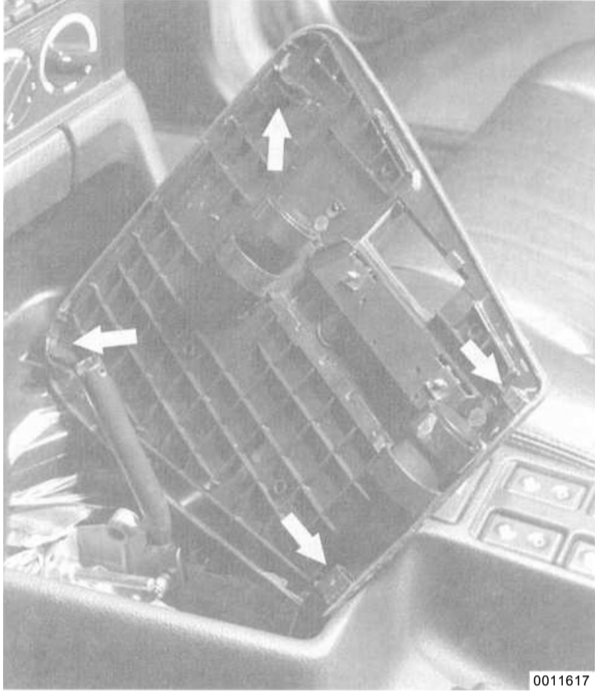
Fig. 7. Console cover shown removed. Pry cover up from front and then lift off rear retaining clips.
