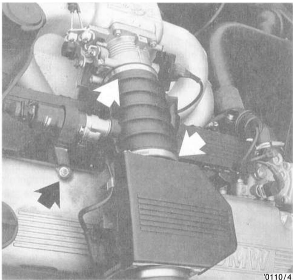
Fig. 34. Disconnect hose clamps and remove idle air control valve mounting bracket (arrows) to remove Intake air boot.
