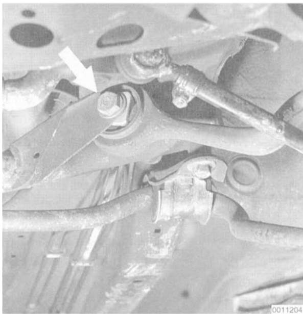
Fig. 15. Thrust arm through-bolt (arrow).
