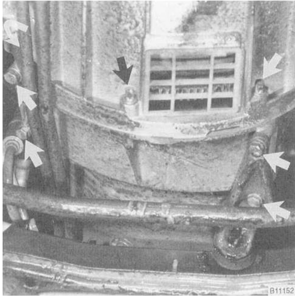
Fig. 4. Bellhousing reinforcement plate mounting bolts (arrows).
