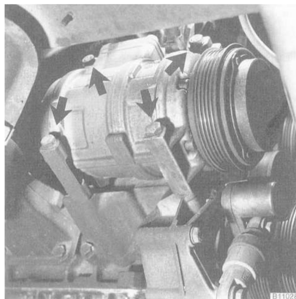
Fig. 20. A/C compressor mounting bolts (arrows)
