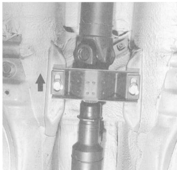
Fig. 8. Preload center bearing toward front 4-6 mm (arrow).
