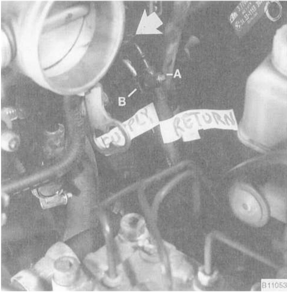
Fig. 14. Fuel return (A) and fuel supply (B) lines at Intake manifold.
