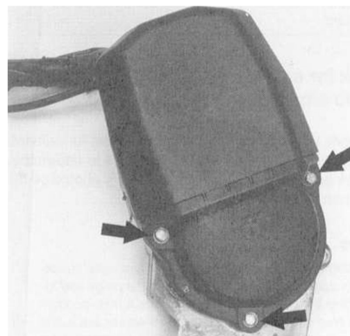
Fig. 5. Distributor cap mounting screws (arrows).
