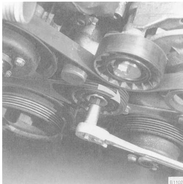
Fig. 21. Poly-ribbed drive belt being removed. Turn 8 mm hex wrench clockwise to relieve belt tension and then slip belt off pulley.
