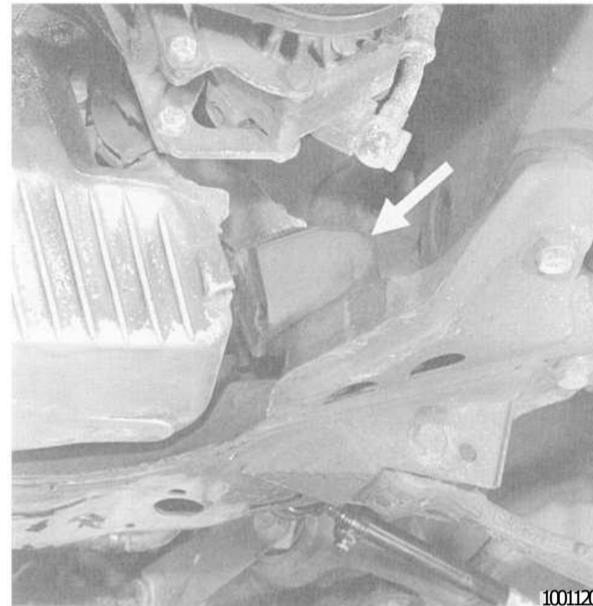
Fig. 17. Left lower engine mount (arrow).
