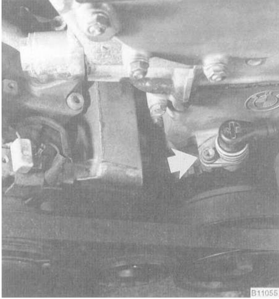
Fig. 17. Reference/speed sensor mounting bolt (arrow).
