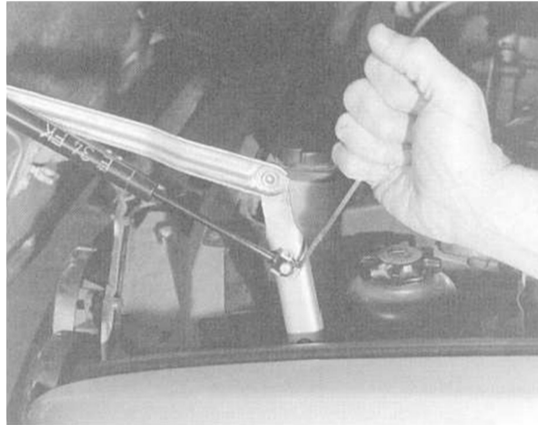
Fig. 10. Hood support strut being removed. Pry clip up while pulling strut from stud.
