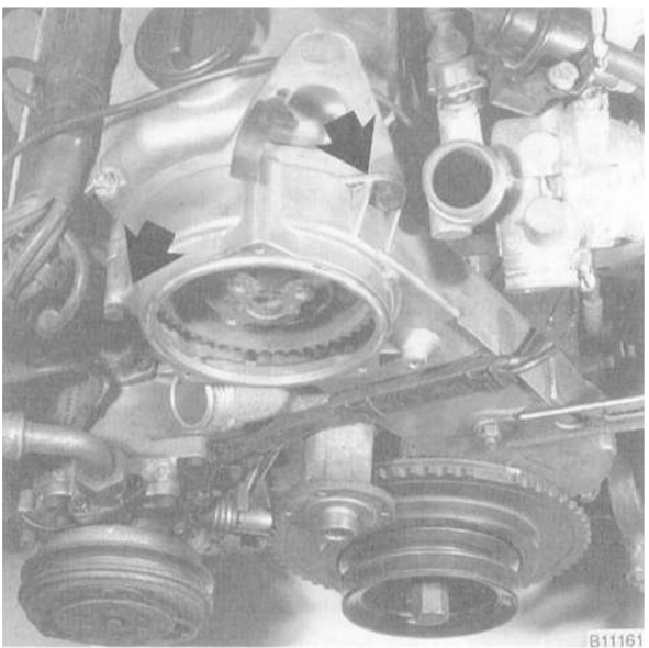
Fig. 3. Upper camshaft drive belt cover mounting bolts (arrows).
