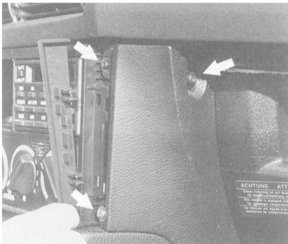
Fig. 4. Plastic trim panel being removed (1991 and later cars only). Trim panel mounting screws shown at arrows.
