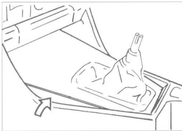
Fig. 2. Remove shift boot cover by prying up at rear (arrow) and then lifting off from front retainers.
