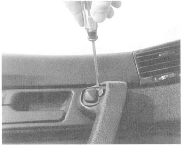
Fig. 8. Outside mirror switch being removed from door arm rest.
