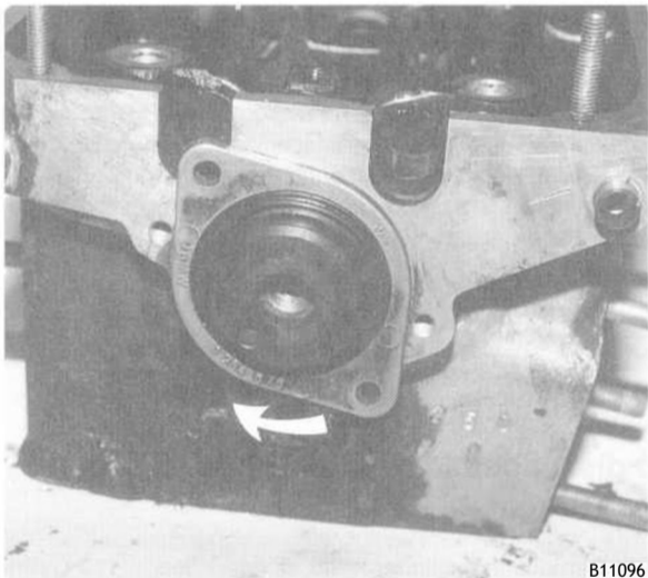
Fig. 18. Camshaft oil seal housing at front of cylinder head. Rotate oil seal carrier during removal ( arrow ).
