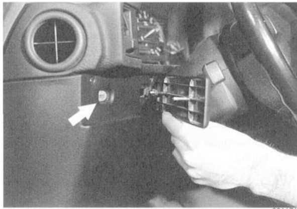
Fig. 12. Lower instrument panel trim cover being removed on cars with SRS airbag. Pry cover out of clip (arrow), then slide cover outwards toward left.
