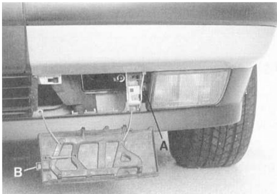
Fig. 6. Fog light retaining screw (A). Remove towing eye cover by depressing locking tab (B) and lifting out cover.
