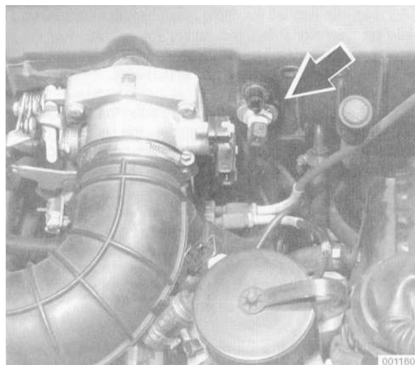
Fig. 7. Intake air temperature sensor location on M50 engine (arrow)
