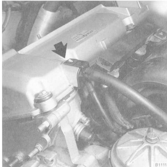
Fig. 3. Crankcase ventilation hose fitting (arrow).
