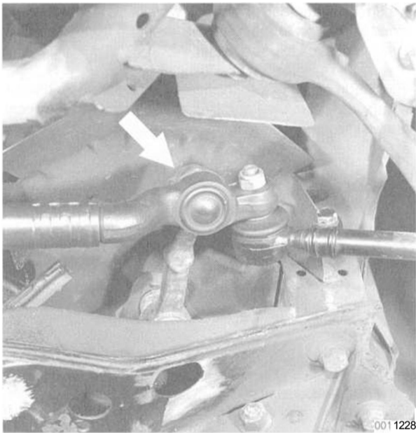
Fig. 8. Idler arm-to-center tie rod self-locking nut (arrow).
