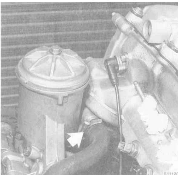
Fig. 6. Coolant hose at oil filter housing (arrow)
